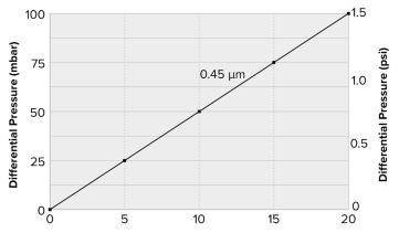
Flow (L/min) for liquid at 20°C (68°F) and 1 cp 10" module
